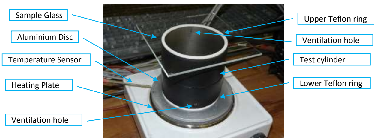
Figure 1: Test device for laboratory testing of outgassing
